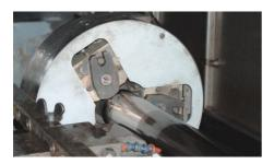
Grinding drivers from Elaso are first class quality products for reliable and profitable driving of parts between centers during cylindrical grinding.
