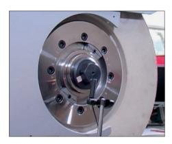
The balancing processor ebm100 calculates the weight positions on the grinding wheel flange for optimum balancing results. Only two weights are needed. Step by step, the user is guided through the balancing run. Each step position is indicated by an LED.
