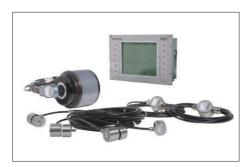
The ebg1500 is a balancing and structure-borne noise system for highest demands. It is used for balancing grinding wheels, to increase production, and to monitor grinding processes. Short production cycles and/or high accuracy requirements are areas where this unit is utilized. The ebg1500 is highly sensitive and is able to recognize within a few micrometers infeed the contact between part and grinding wheel. This reduces the air grinding time considerably.
