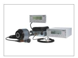
The eb4500 balancing controller offers either fully automatic or manual balancing of grinding wheels. A balancing head, which is either built onto the spindle end or within a hollow spindle, is manipulated by the controller. Vibrations from the grinding wheel are recorded with a vibration transducer and displayed on the controller. A collector connects the balancing electronics with the rotating balancing head. Brush type or maintenance-free nocontact collectors are available.
