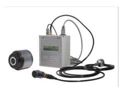
The eb2000 offers either manual or fully automatic balancing of grinding wheels. A balancing head, which is either built onto the grinding spindle end or within a hollow spindle, is controlled by a control unit. Vibrations from the grinding wheel are recorded with a vibration transducer and displayed on the controller. A collector connects the balancing electronics with the rotating balancing head. Brush type or maintenance-free no-contact collectors are available.
